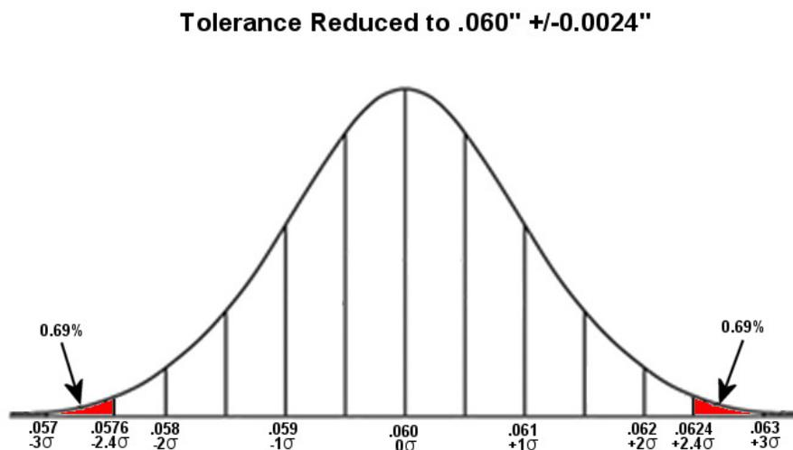
The percentage of parts represented by the shaded area under the curve between  $2.4 \sigma$  and  $3 \sigma$  is the ambiguity area, where good parts could be falsely rejected.
