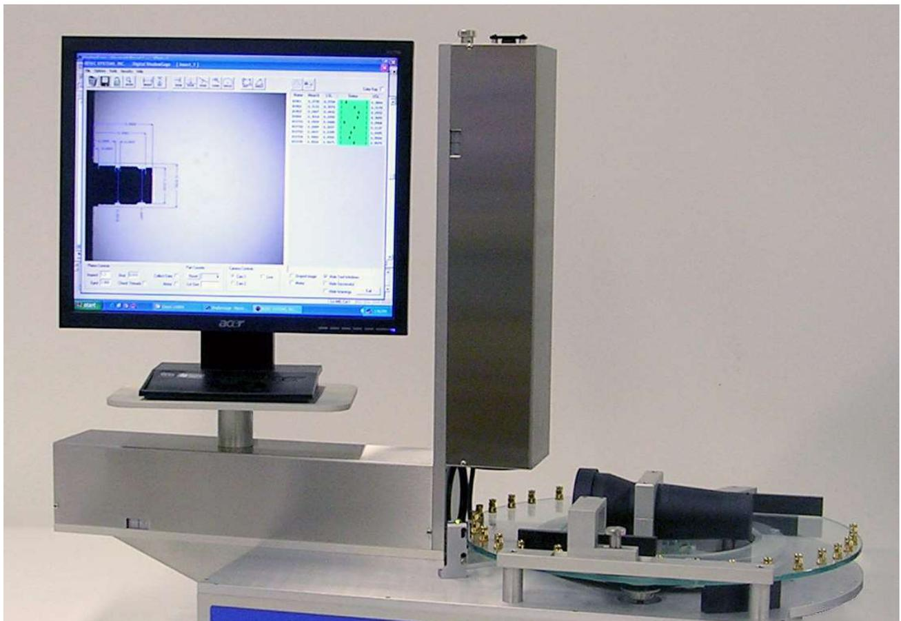
Software is used to create and edit inspection programs as well as set operational parameters and calibrate equipment. A screen displays the parts' image with the overlaid measurements, and inspection programs are created directly over the interactive image. For further flexibility, the software is used to create and edit inspection programs as well as set operational parameters and
